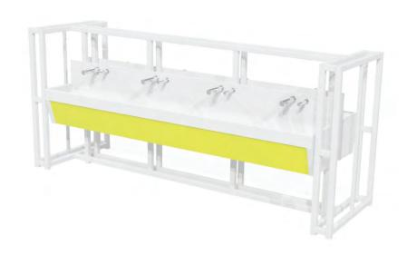
The Modular Island Unit is designed to provide a safe structural half height support frame to mount washtrough onto. When washtroughs are required to be fitted in the middle of a room or projecting out from a wall, the steel modular island unit can be bolted to the ground. The void between the two troughs is designed to hide all pipework and can contain the ONVO multifeed soap container.
