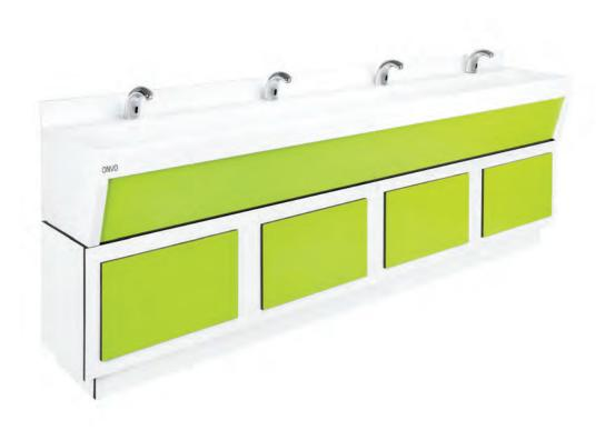
The ONVO Latherwash 2D with Modular Frame is designed for installations where the pipework below the trough needs to be concealed or where the trough cannot be cantilevered off the wall. The taps are mounted onto the deck of the trough and therefore no void is required behind. The Latherwash 2D with Modular Frame is very slim, only projecting 400mm from the wall.
